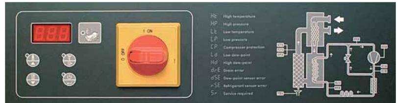
The multifunction SmartControl provides a versatile platform for user interface and SmartSave Cycling (if enabled). The innovative SmartSave (patent pending) Cycling Control continuously monitors the demand placed on the dryer. At conditions of low demand the refrigerant compressor is cycled off to save energy. A sophisticated algorithm continuously adapts the operation of the dryer for optimum energy efficiency while minimizing the dewpoint spikes common to traditional thermal mass dryers.
